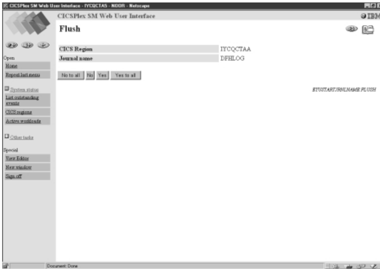
Figure 18. Confirmation panel for flushing the DFHLOG journal
